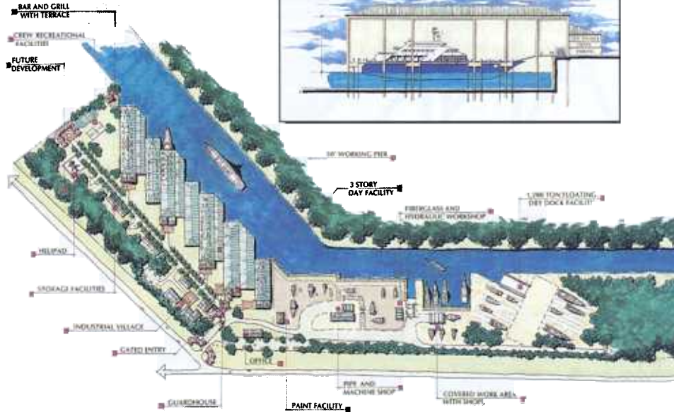
The final build-out of the Grand Bahama facility is shown in this site plan.
